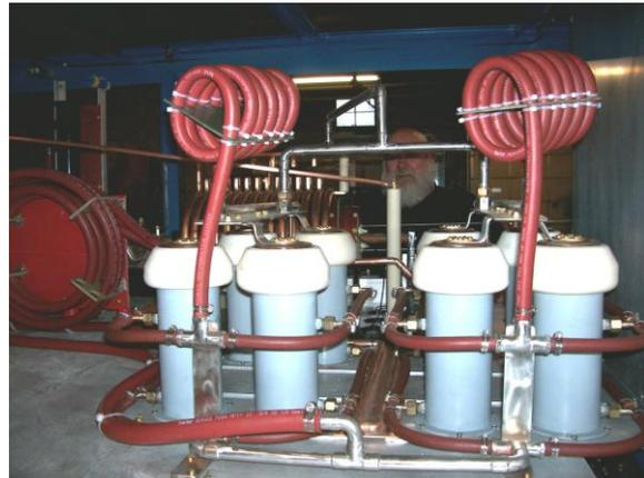
The BW1185J2 triode is rated to work up to 30 Mhz. Typically they operate on a frequency of 455 khz in these machines and run at just over 50% over-all output to input. The power output limit of 125 KW in the unit shown in the picture is because of plate transformer ratings, the tube itself is
